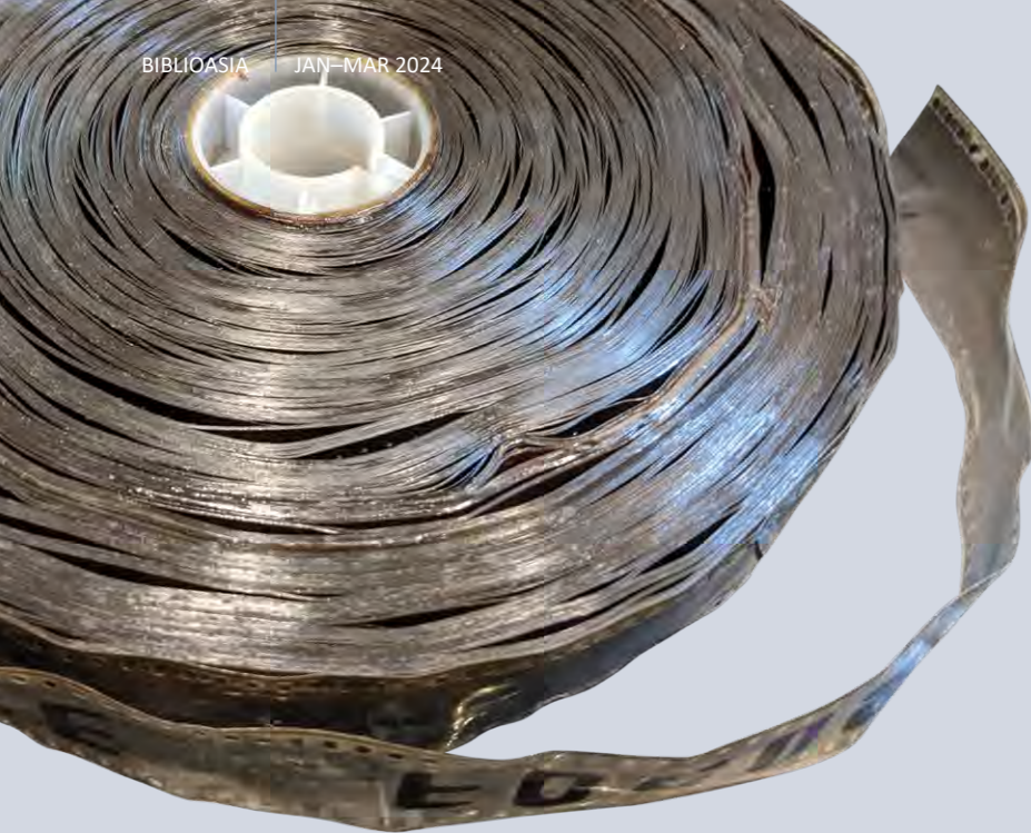
Most of the film base of Dharmasena Pathiraja's Bambaru Avith had softened and the emulsion had become sticky. Warpage and shrinkage were observed in every reel with numerous adhesive stains and perforation tears. Courtesy of Asian Film Archive.
